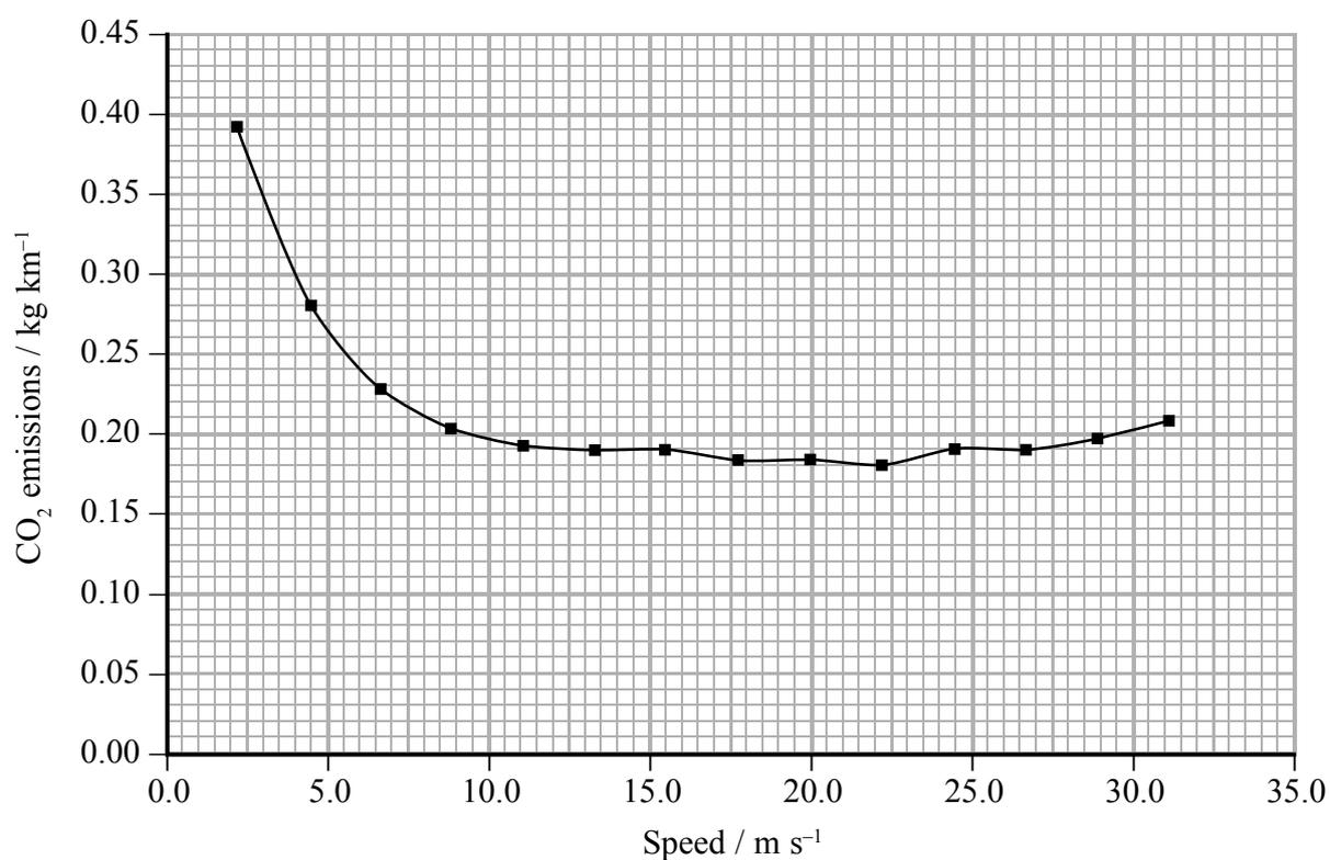
During a 10 minute journey a cyclist, travelling at  $5 \text{ m s}^{-1}$ , has an average of three cars queuing behind him. The cars would otherwise be travelling at  $18 \text{ m s}^{-1}$ . The cars emit more carbon dioxide because they are travelling slowly.
